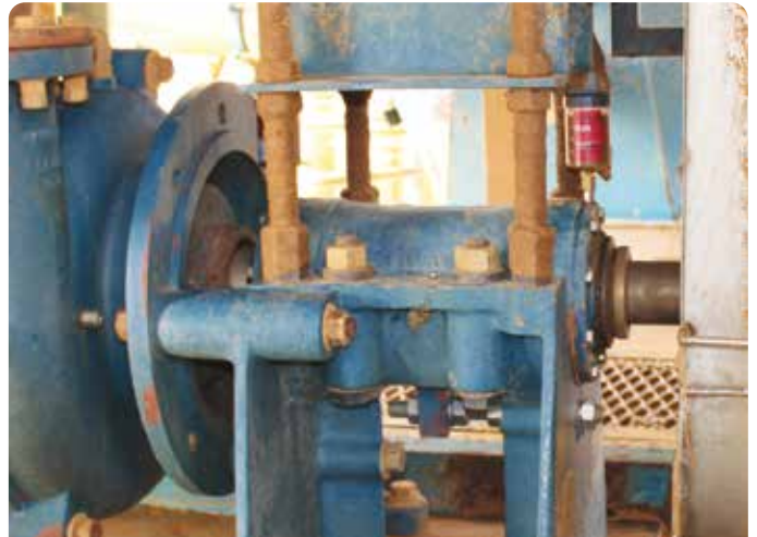
Application Horizontal slurry pump labyrinth seals Lubricator perma FLEX125 Installation kit Direct mount
