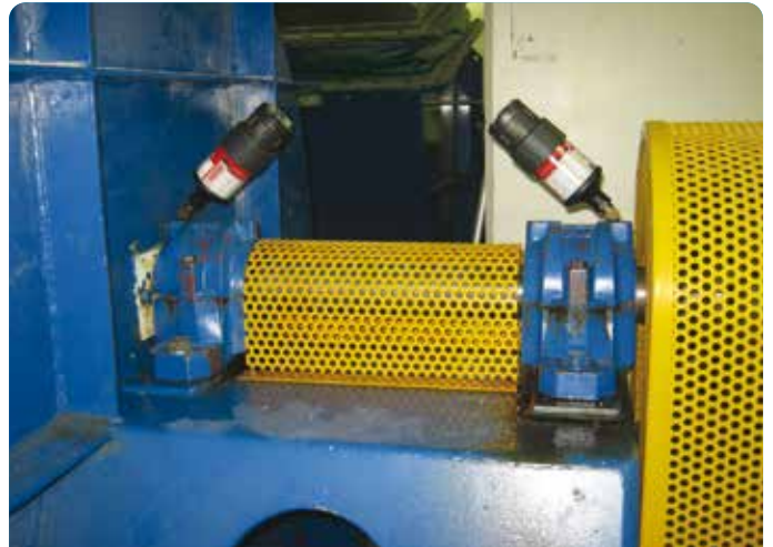
Application Fan support bearings Lubricator perma STAR VARIO M120 Installation kit Direct mount
