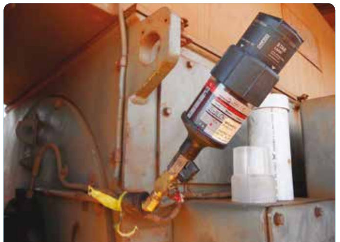
Application Electric motor Lubricator perma STAR VARIO M120 Installation kit Direct mount
